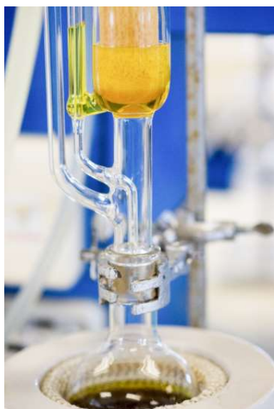
Fig. (2). The crude extracts are extracted using the soxhlet method.
